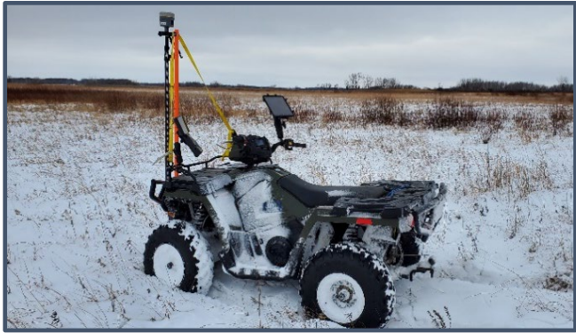
Figure 1 Topography survey are done to identify potential wetland restorations and enhancements and provide data for construction planning.
