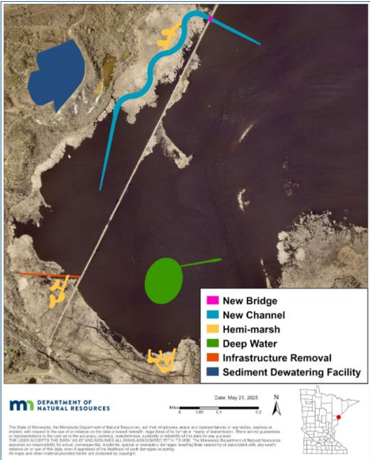
Figure 1. Illustration of habitat restoration features included in the 95% design plans for Mud Lake.
